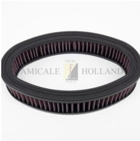
AIR FILTER ELEMENT TY7/TY8 (ALTERNATIVE) WASHABLE
